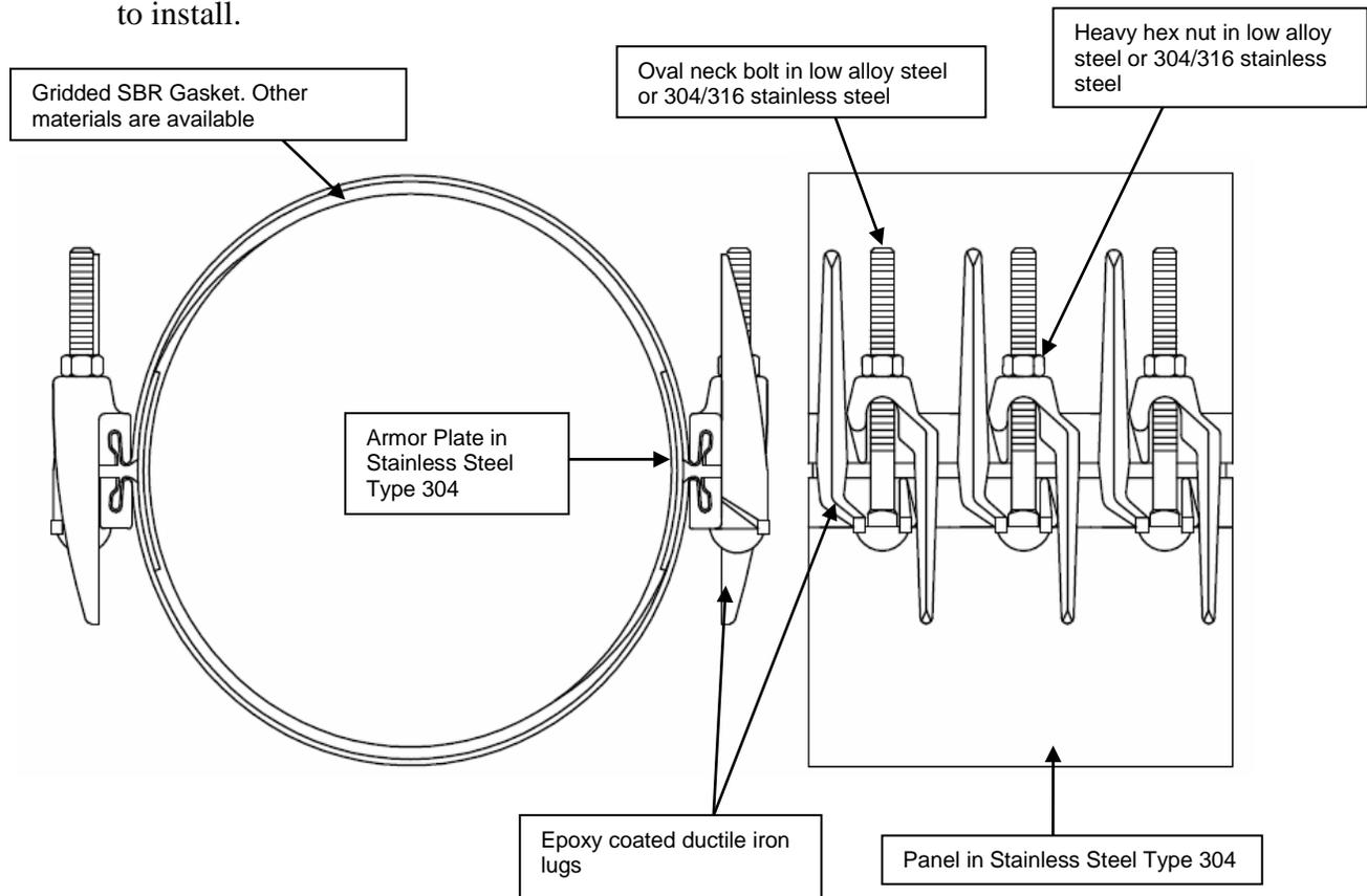
\*The pressure rating depends on the installation and the extent of damage of the pipe as well as the condition of the pipe.
