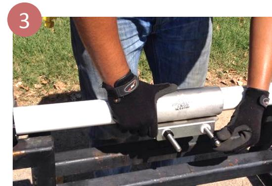
3 Tuck the gasket flap in place, close the bolt lug, engage the centermost bolt(s) and finger tighten. NOTE: using the palm of your hand, squeeze the end of the clamp fingers and the top of the stud lug to bring stud bolt and fingers parallel.
