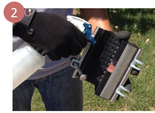
2 Loosen the nut to the end of the bolt and open the clamp. Do not disassemble. Lubricate pipe and gasket with soap/water solution.
