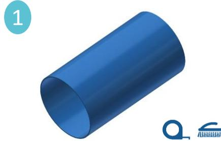
1 Thoroughly clean the pipe where the saddle will be installed. There should be no foreign debris between the gasket and the pipe surface. Double check OD so that it matches range on your saddle.
