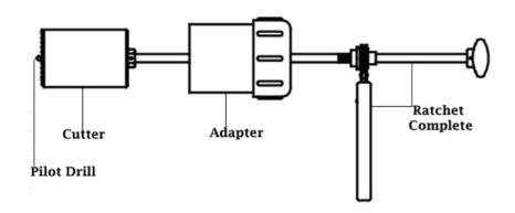
\*Complete units consist of Sewer Cutter, Ratchet, Shaft, and Adapter.
