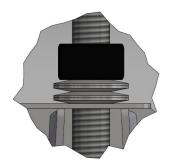
Waterworks pipes can experience changes temperature and pressure depending on the field High-Density conditions. Polyethylene **Pipe** possesses mechanical and thermal properties that cause the expansion or contraction of the pipe because of these changes. 3122AS-PE with spring washers design will support those possible pipe changes without compromising the tightness of the clamp.
