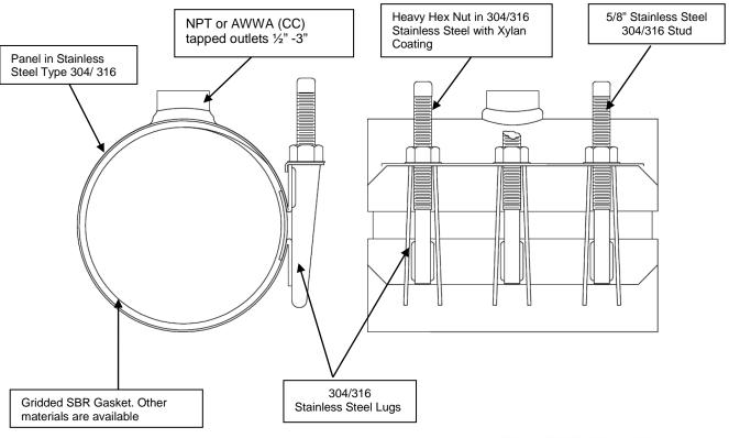
\*The pressure rating depends on the installation and the extent of damage of the pipe as well as the condition of the pipe.
