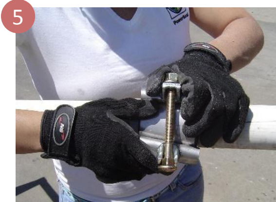
Once the clamp is in the right position, fit the bolt head on the hook of the lug and start tightening the nut by hand.
