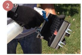
Loosen the nut to the end of the bolt and open the clamp. Do not disassemble. Lubricate pipe and gasket with soap/water solution.
