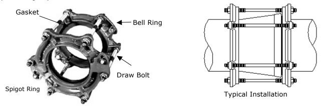
**3. INSTALL BELL RING:** Assemble one set of ring segments behind the bell. Adjust ring to suitable diameter, and lock ring segments into position by tightening nuts.
