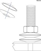
High Density Polyethylene Pipe (HDPE) has lower modules of elasticity and higher coefficient of thermal expansion than other pipe materials. These properties cause HDPE pipe to expand and contract due to changes in temperature and/or pressure much more than other types of more common waterworks pipe. The 3414AS-PE saddle with spring washers design will support those possible pipe changes without compromising the tightness of the saddle.
