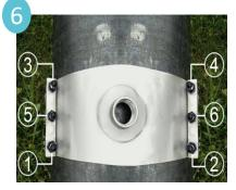
Tighten maintaining an even gap distance between the bolt lugs on both sides of the saddle. 25 ft-lb increments recommended.
