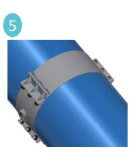
If necessary, to reposition loosen nuts prior to moving saddle and then re-torque. Hydrostatically pressure test the saddle before tapping the pipe.
