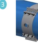
Install bolts, spring washers, (see figure 1) and nuts through lugs as shown. Tighten maintaining an even gap distance between the bolt lugs on all three sides of the saddle. 25ft-lb increments recommended.
