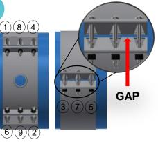
Tighten bolts in sequence, beginning at the ends of the saddle and alternating on all three sides. The gap between the lugs must be equal distance when saddle is fully tightened.
