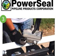
Loosen nuts until flush with top of studs, and place saddle around pipe.
