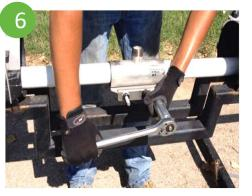
Gradually torque nuts 50 to 70 ft/lbs to form a gasket seal. Do not over torque as it will not increase sealing ability, but may cause plastic pipe failure.
