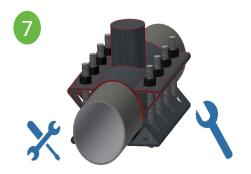
Tighten bolts in sequence, beginning at the ends of the sleeve and alternating on both sides. The gap between the two halves must be of equal distance when sleeve is fully tightened.
