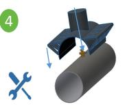
Once the main stop is closed, remove the copper tubing for the corporation stop if still attached. Place the encapsulating section of the sleeve over the corporation stop and onto the pipe. Make sure the tapered gaskets are smooth against the pipe.
