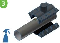
Lubricate pipe and gasket with soap/water solution. **Do not use grease or pipe lubricant.**
