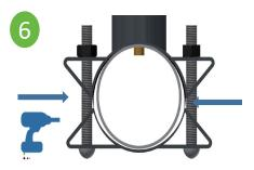
Install bolts, washers and nuts. Tighten maintaining an even gap distance between the bolt lugs on both sides of the sleeve; i.e. 25 ftlb increments. Nuts must be tighten in the order shown in the image.
