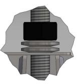
Waterworks pipes can experience changes due to temperature and pressure depending on the field conditions. High-Density Polyethylene Pipe (HDPE) possess mechanical and thermal properties that causes the expansion or contraction of the pipe because of these changes. Repair clamps with spring washers design will support those possible pipe changes without compromising the tightness of the sleeve.
