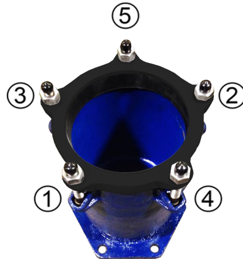
Nuts must be tighten in the order shown in the image.
