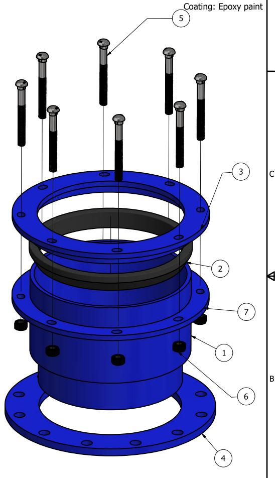
Unless otherwise stated all dimensions are in inches. Flexible couplings do not provide against pull out of pipe
