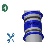
Position the center barrel over the pipe (position barrel within the two reference marks) and attach gasket & gland assembly at both ends of the center barrel.
