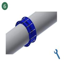
Pressurize the line, check the leakage, and re-torque if necessary. \*Pressure test all joints before covering coupling.
