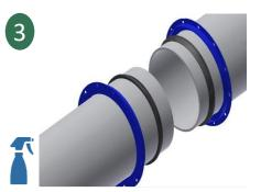
Lubricate pipe and gasket with soap/water solution and begin installation by placing one gland and one fully lubricated gasket over each pipe end.
