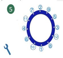
Install and evenly tighten bolts and nuts to recommended torque alternating between opposite sides of coupling as shown in the image.
