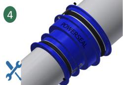
Position the center barrel over the pipe (position barrel within the two reference marks) and attach gasket & gland assembly at both ends of the center barrel with the bolt head on the inside and the nut on the gland side.
