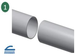
Thoroughly clean the pipe surface, and inspect the area where the coupling will be installed for flaws, i.e., gouges, protrusions, excessive corrosion, etc. Irregular surfaces should be avoided to assure maximum gasket sealing.
