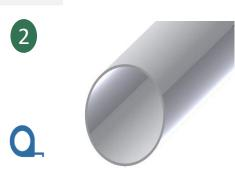
Check the main outside diameter (OD) and confirm that it falls within the coupling pipe OD range. Place a reference mark on both pipe ends to ensure the coupling will be centered. There should be a minimum of 2" of pipe insertion per coupling end.
