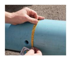
Measure the pipe in a quick and easy way. Wrap the O.D. Tape around the pipe and you will have your exact O.D.
