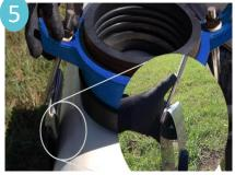
free end between strap and pipe. (On small pipe, it may be necessary to fold loose end twice).
