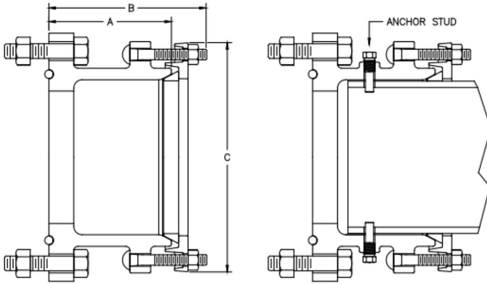
**Note:** Protection against possible pull out of pipe ends is not provided with cast couplings unless pipe is restrained.
