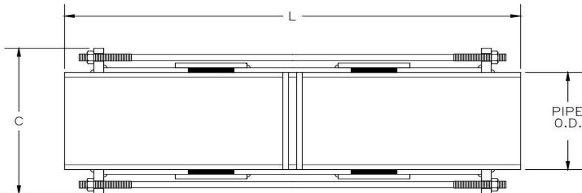
**DOUBLE END WITH LIMIT RODS (DELRL)**
