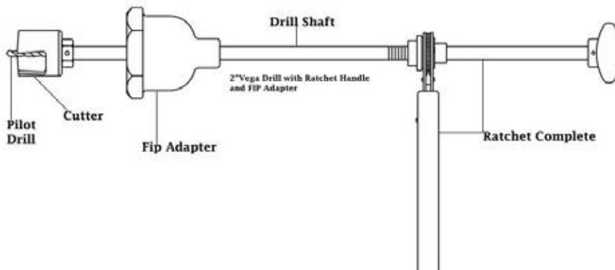
\*Complete units consist of Drill, Drive Mechanism, and type of adapter specified.
