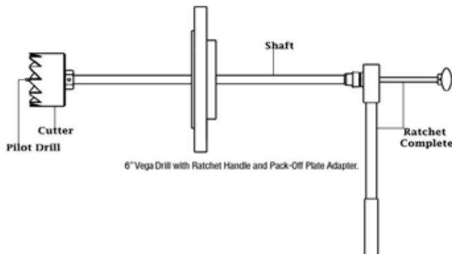
6" Vega Drill with Ratchet Handle and Pack-Off Plate Adapter.
