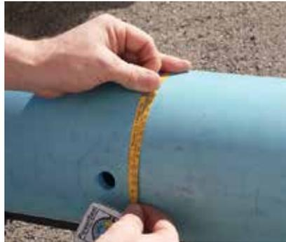
Measure the pipe in a quick and easy way. Wrap the O.D. Tape around the pipe and you will have your exact O.D.
