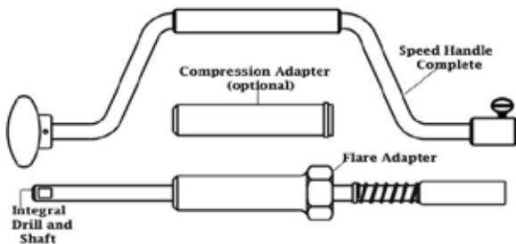
3/4" C900 Vega Drill with Speed Handle and Flare Adapter.
