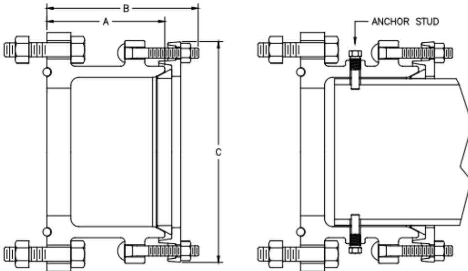
**Note:** Protection against possible pull out of pipe ends is not provided with cast couplings unless pipe is restrained. Pipe diameters less than IPS/STEEL rated up to 50 psi work pressure.
