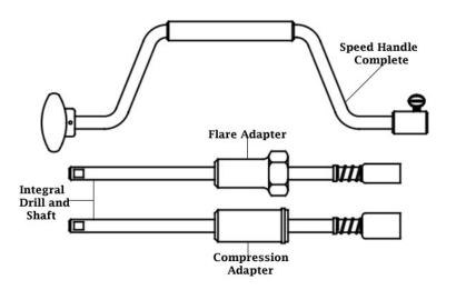
3/4" and 1" Combination Vega Drills with Speed Handle, 3/4" Flare Adapter and 1" Compression Adapter.
