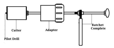
4" Sewer Vega Drill with Ratchet Handle and Guide Adapter.
