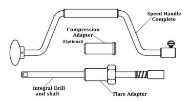
\*Complete units consist of Drill, Drive Mechanism, and type of adapter specified. \*The Vega Drill Speed Handle Drive Mechanism is available only on 3/4" & 1" units. \*The 1 1/2" & 2" units are furnished with Female Iron Pipe (FIP) threaded Adapters unless otherwise specified.
