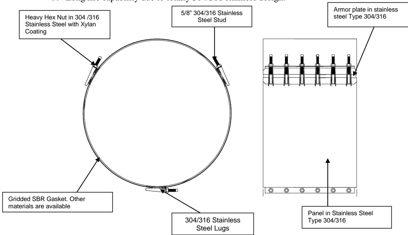
\*The pressure rating depends on the installation and the extent of damage of the pipe as well as the condition of the pipe.
