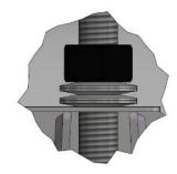
Waterworks pipes can experience changes due to temperature and pressure depending on the field conditions. **High-Density** Polyethylene Pipe (HDPE) possess mechanical and thermal properties that causes the expansion or contraction of the pipe because of these changes. Repair clamps with spring washers design will support those possible pipe changes without compromising the tightness of the saddle.
