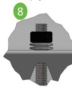
Tighten both top and bottom bolts evenly, alternating from one side of the sleeve to the other. Torque according to the specifications. Wait approximately 5 minutes to allow the gasket to fully compress and then re-tighten bolts. The spring washers must be stacked in series as shown in picture.
