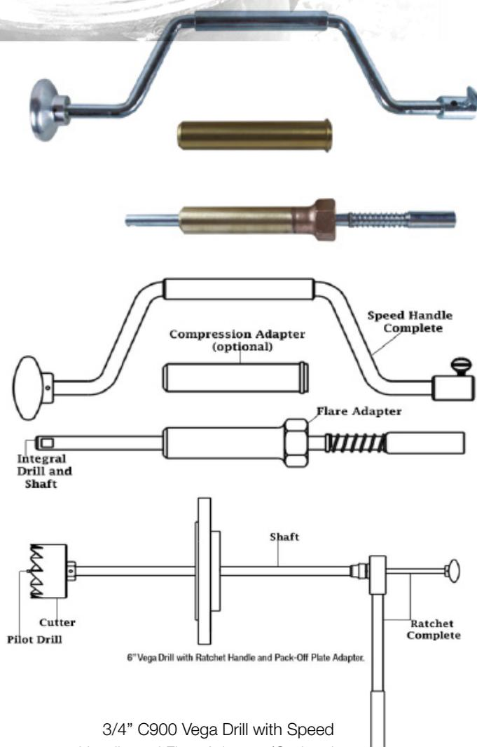
3/4" C900 Vega Drill with Speed Handle and Flare Adapter. (Optional Compression Adapter also shown.)
