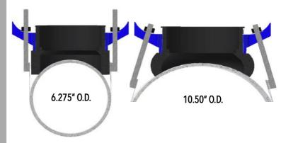
Same sewer saddle installed on different outside diameters of pipes
